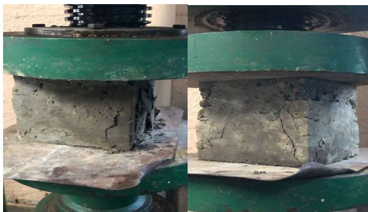
Figure 4: Compressive strength test of cement concrete cube
