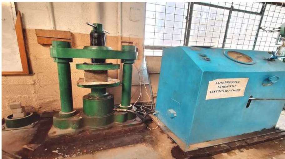
Figure 3: Compressive strength testing machine
